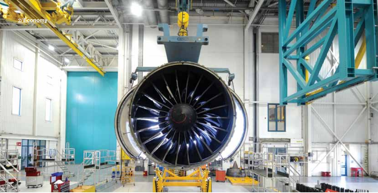
A GE90 engine being serviced at the Nantgarw aircraft maintenance plant – the biggest aero-engine in use world-wide, developed exclusively for the Boeing 777.
