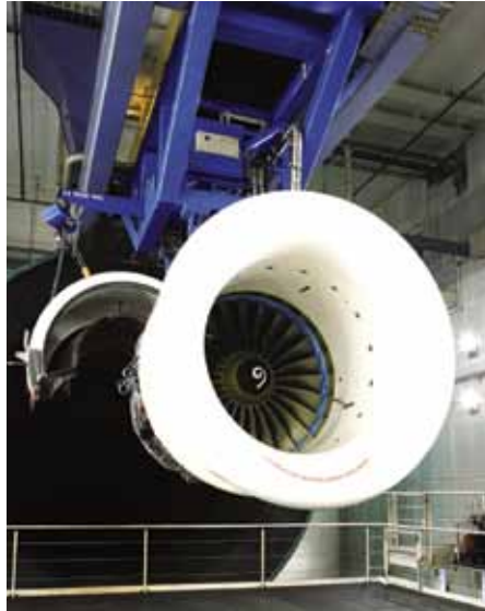
A CFM56 engine being tested at Nantgarw. It is the world's most popular aero-engine, with 20,000 currently in service worldwide.
