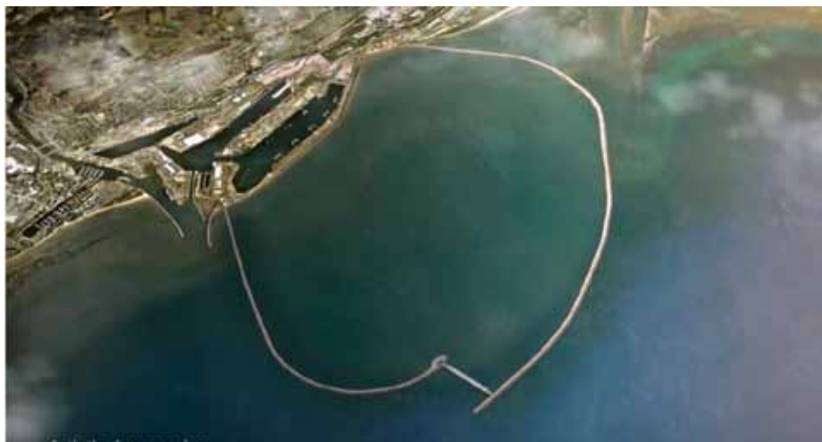
Swansea Bay Tidal Lagoon is a man-made seawall impounding a 12 square kilometre area of water. Power is generated by creating a 'head' of water – the difference in water level between the inside and outside of the lagoon – and channelling the resulting flow through low-head hydro turbines.
